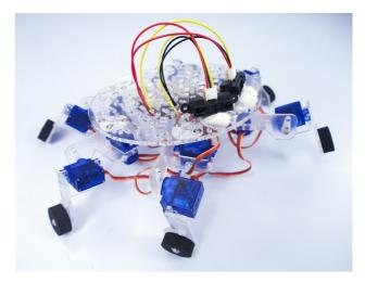
Figure 8. Sparkfun 12 servo hexapod robot with IR range sensors
