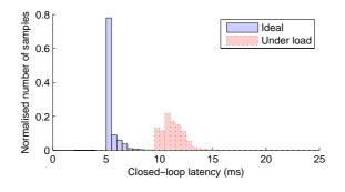
**Figure 5**. Closed-loop latency evaluation (distribution of approximately 50,000 samples)
