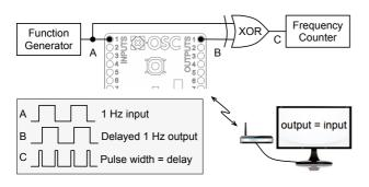
**Figure 4**. Experimental setup for evaluation of closed-loop latency
