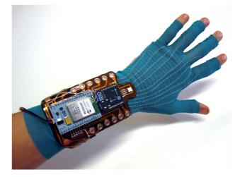
**Figure 6**. The x-OSC data glove, incorporating an IMU, RGB LED, vibration motors and e-textile flex sensors
