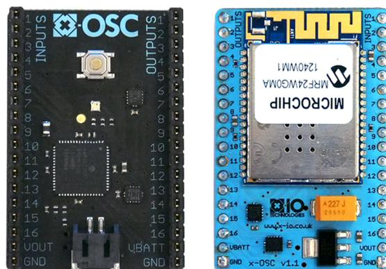
**Figure 2.** x-OSC board top (left) and bottom (right), size:  $31 \times 47$  mm
