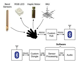
Figure 1. Data flow diagram for one of two data gloves in the current version of *The Gloves*
