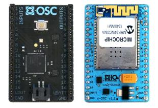
Figure 2. x-OSC board top (left) and bottom (right), size:  $31 \times 47 \text{ mm}$
