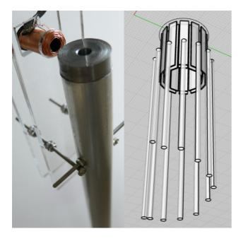
**Figure 7**. Solar wind chime: top of aluminium tube with electromagnet (left) and solar wind chime assembly design (right)
